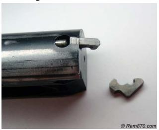
Machined extractor is one of the must-have upgrades for your Remington 870. It insures reliable extraction of fired shells. Police version of the Remington 870 utilizes non-MIM extractor too because it is more reliable.
