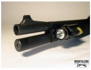
Streamlight TLR-2 Flashlight/Laser combo. I have installed it using CDM Gear BMT clamp with picatinny rail. I think this is the best way to attach Streamlight TLR-2 or Streamlight TLR-1 to Remington 870. I really like this flashlight/laser combo, it is lightweight and easily attaches to a rail. TLR-2 is low profile and doesn't stick out much. Streamlight TLR-1 which doesn't have laser is even smaller. Stremalight TLR-2 has lots of great features.
